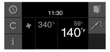
5 The appliance heats with the set heating function. The current core temperature is displayed and, under it, the set core temperature. You can change the set core temperatur at any time. A signal sounds when the set core temperature in the food has been reached. The cooking mode is ended automatically. Confirm with  $\checkmark$  and turn the program selection to 0.
